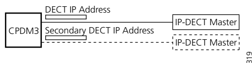
Figure 28. Communication with the IP-DECT system is done over a LAN
